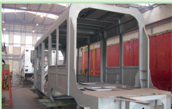
Fabrication of Tango light rail carriages in the workshop (Photo: ThyssenKrupp Nirosta)
