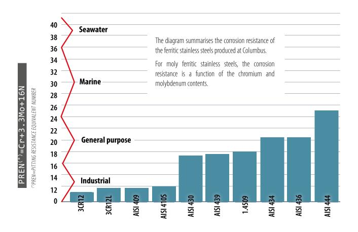
In common with other ferritic stainless steels, the **moly ferritics** are not susceptible to Stress Corrosion Cracking (SCC). 434 and 436 have similar general corrosion resistance to 430.
