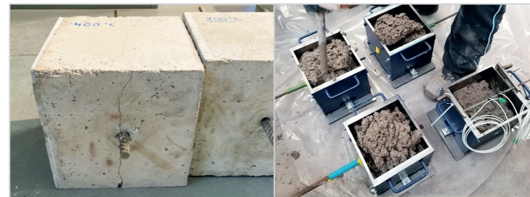
Fig. 2 Adhesion test specimens after exposure to high temperatures. Self-manufactured.
