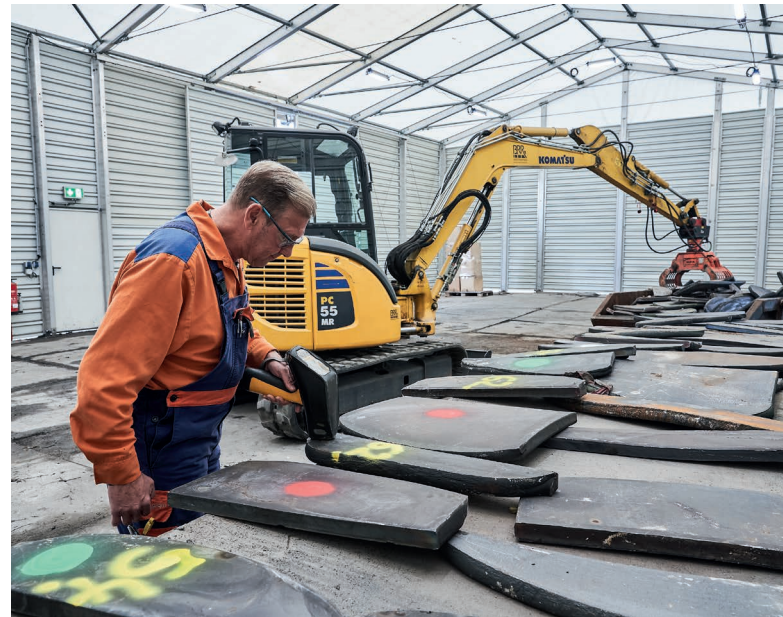
Figure 2: Analysis of scrap pieces by means of a spectrometer
