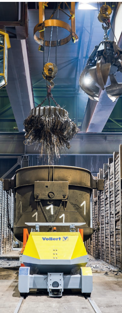
Figure 1: Charging of recycling materials during preparation of a melt
